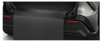
The rear bumper protection apron is fixed to the trunk deck with velcro. It protects the rear bumper when unfolded.
