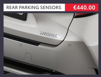
Rear parking sensor system with 4 ultrasonic sensors and an acoustic warning.
