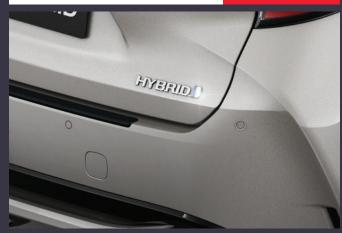
Rear parking sensor system with 4 ultrasonic sensors and an acoustic warning. The system works with 4 sensors.
