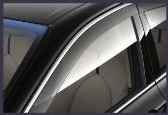
Wind deflectors are ideal if you like to drive with the windows open. They are custom designed to match the aerodynamic contours of your vehicle and work by diverting airflow to ensure that you and your passengers are not troubled by excessive wind movement and noise.
