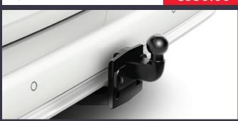
Flanged ISO tow ball for flanged towing hitch (SWB & LWB).
